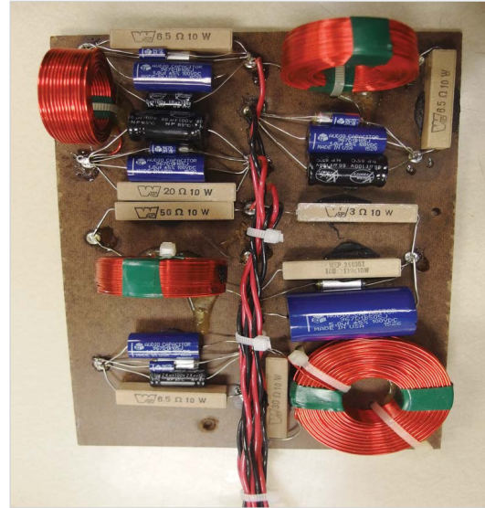
Figure 10: Typical Speaker Crossover Network
